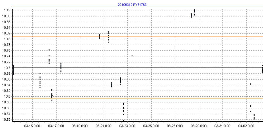
Figure 2 Data screening showing +/- 1% and +/- 2% bands, note the morning and afternoon data clusters as the airmass is passing through the nominal  $AM_a \sim 1.5$  value
