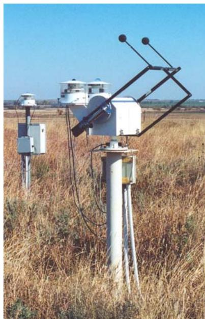
Figure 2. Unshaded pyranometer (Left) for GH measurement, shaded pyranometer and pyrgeometer (on solar tracker horizontal platform) for DIFF and downwelling longwave (infrared – for atmospheric science study), and pyrhelometer (on sided of solar tracker) for DNI measurements at the DOE/ARM Southern Great Plains station near Lamont, Oklahoma.
