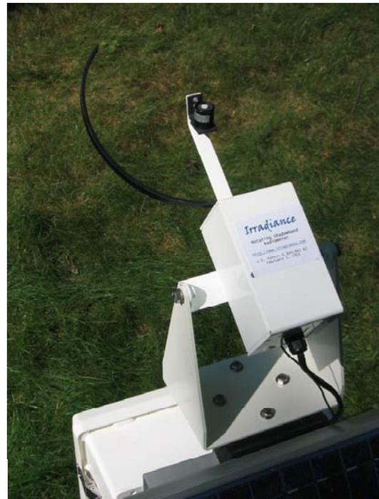
Figure 1 *Irradiance* RSR-2 head unit and solar resource measurement system.
