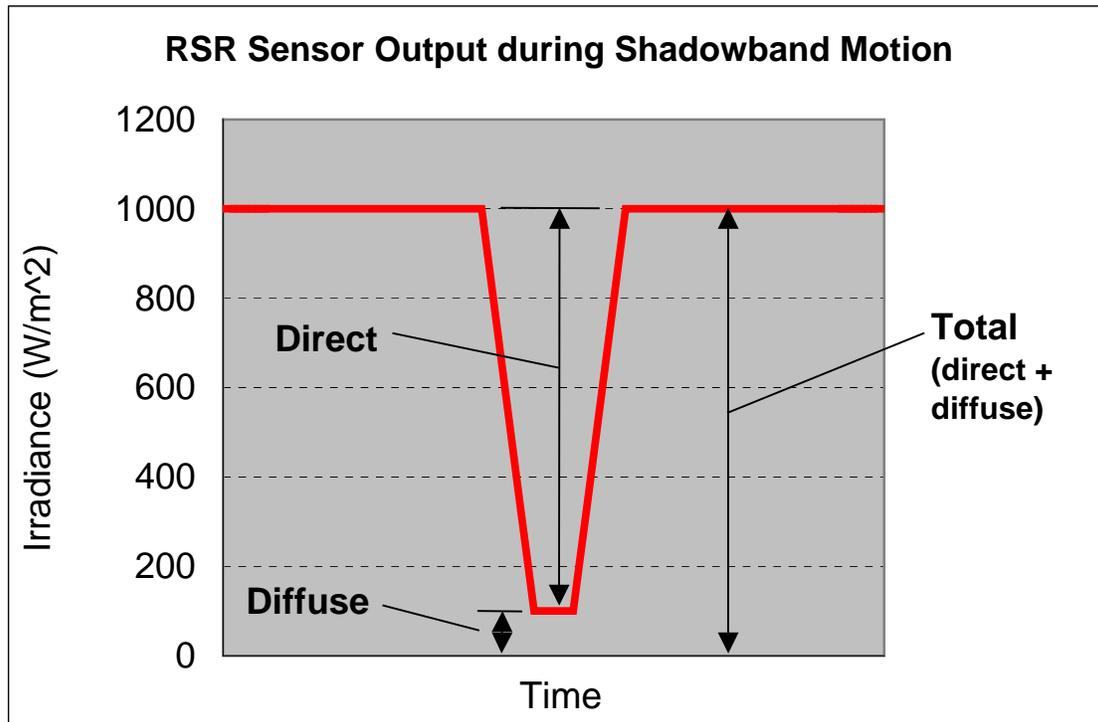
The Irradiance RSR2 uses a single light sensor (pyranometer) to measure the total and diffuse irradiance, allowing accurate derivation of the direct irradiance. These terms are related by:
