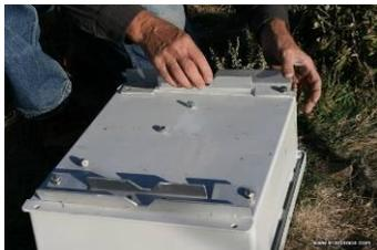
C. Use the U-Bolts to attach the enclosure brackets to the center tube. Attach it on the north side of the tripod, below the intersection of the leg and the center pipe.
