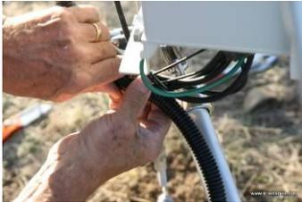
vi. Attach the loose wires into the datalogger; plug the cable into the motor controller.
