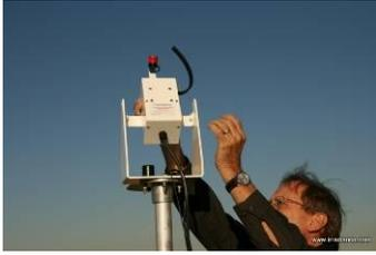
vi. Tighten the screws and level the sensor(s); ***remove the protective red cap!***
