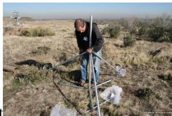
iii. Locate the tripod anchor point
